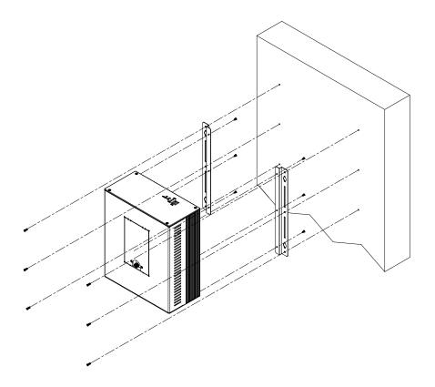
Using attached mounting rail, you can install AMI400 on wood, drywall surface over studs, or a solid concrete or metal plane. Ensure the installer uses at least four M4 length 8mm screws to secure the system on wall. Six M4 length 8mm screws are recommended to secure the system on wall.
